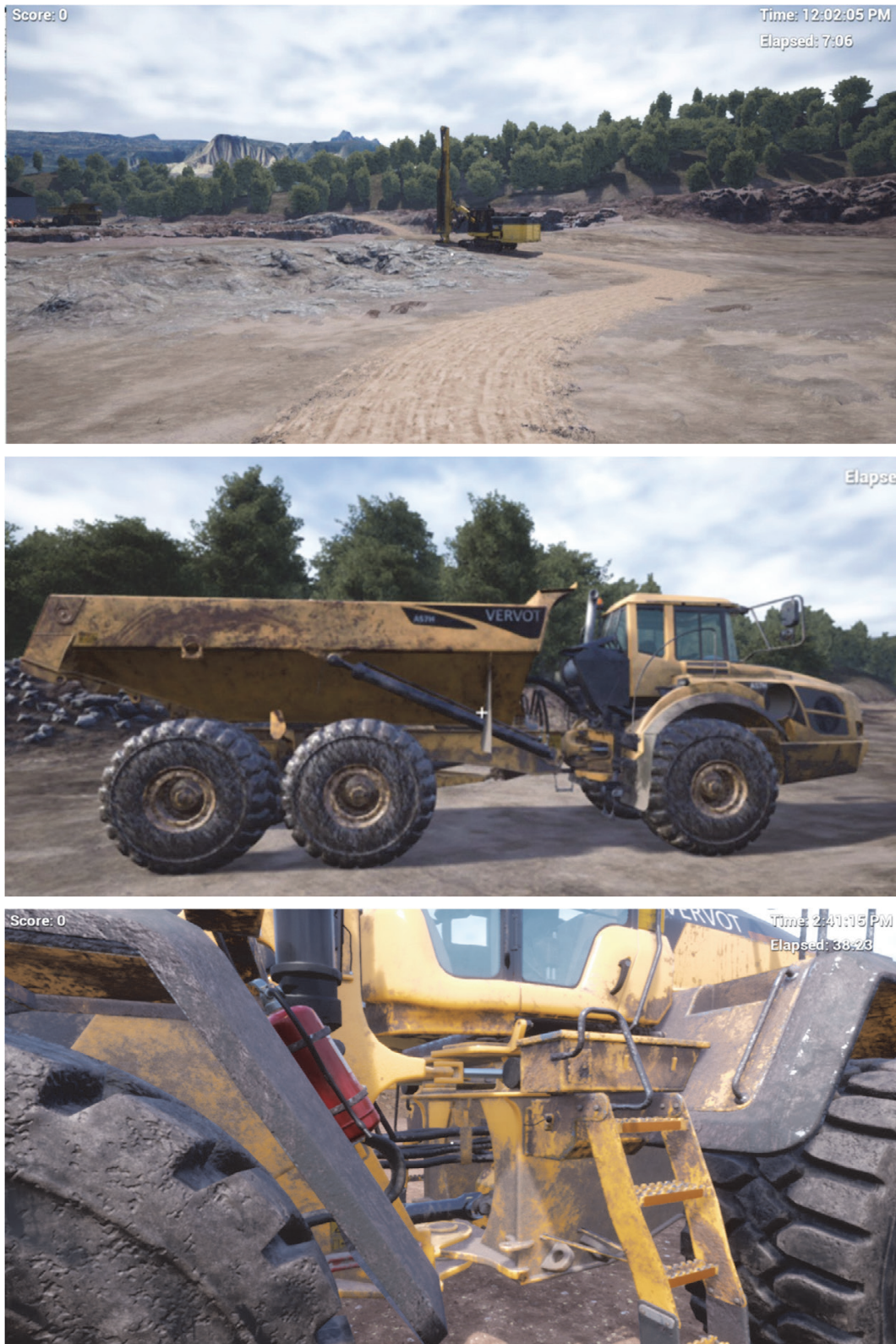
Figure 6. Limestone quarry. Virtual environment features high-detail working faces, travelways, and berms, with user-playable equipment including haulage and loaders.
