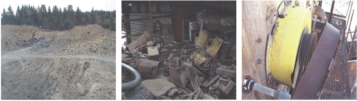
Figure 4. Example hazards in HHD . Left: Berms and guardrails; Center: Housekeeping; Right: Guarding of moving machine parts. (Photos courtesy D. Brown, Mine Safety Assistance, LLC.)
