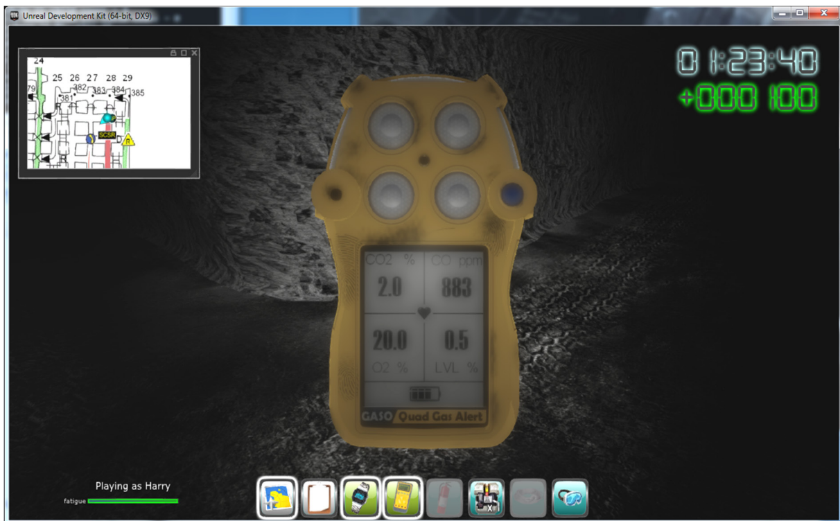
Figure 12. A gas multi-meter. Users must interpret gas readings and manage their time on apparatus. Gas levels become increasingly lethal and breathing apparatus will expire after designated usage times.
